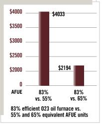
This chart depicts potential energy savings you can expect from the 023 furnace versus older furnaces with lower efficiency ratings. Criteria used in this example are 2,000 full-load heating hours, with a 80,000-Btuh heating design load and \$1.90 per gallon for oil. Your actual savings will vary depending on the weather, local fuel rates and your lifestyle.
